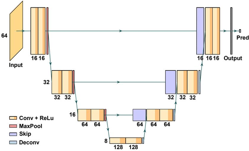
Fig. 3. Illustration of our u-net layout, observe that skip connections and up/down sampling allow the u-net to handle time-series data and perform analysis of data at different frequency levels.
