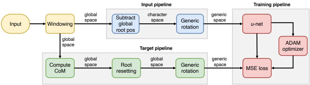
Fig. 2. Input data preprocessing pipeline for motion capture data imported from Rokoko’s Motion Library and targets for training a neural network, u-net, to predict center of mass positions given a time-window of relative joint data input.
