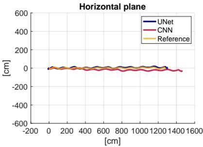
Fig. 7. Top view of a trajectory of a character walking in a straight line. Notice how the u-net estimate is close to the reference while the CNN shows significant drift.
